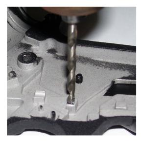
4. Do NOT drill past the lower ledge. This will leave enough room so you don't drill all the way through the body. Bore right receiver half out with 1/4" bit if needed. Remove any burrs or excess material with a small file if necessary.
